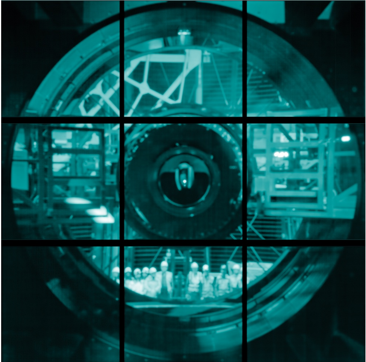
FIGURE 8: In one of the early images taken with Rubin's 144-megapixel test camera, Rubin staff gathered for a group photo inside the observatory dome, with the Simonyi Survey Telescope pointed at horizon. This "pinhole" image was created using the camera's sensors but without using lenses or mirrors to focus light. Instead of forming a detailed, zoomed-in picture, this technique gives a soft, unfocused image. The visible grid pattern of the camera's sensor array overlays the image. Image and caption source: https://rubinobservatory.org/gallery/
