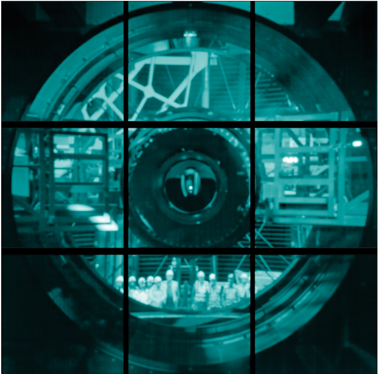
FIGURE 6: In one of the early images taken with Rubin's 144-megapixel test camera, Rubin staff gathered for a group photo inside the observatory dome, with the Simonyi Survey Telescope pointed at horizon. This "pinhole" image was created using the camera's sensors but without using lenses or mirrors to focus light. Instead of forming a detailed, zoomed-in picture, this technique gives a soft, unfocused image. The visible grid pattern of the camera's sensor array overlays the image. Image and caption source: https://rubinobservatory.org/gallery/
